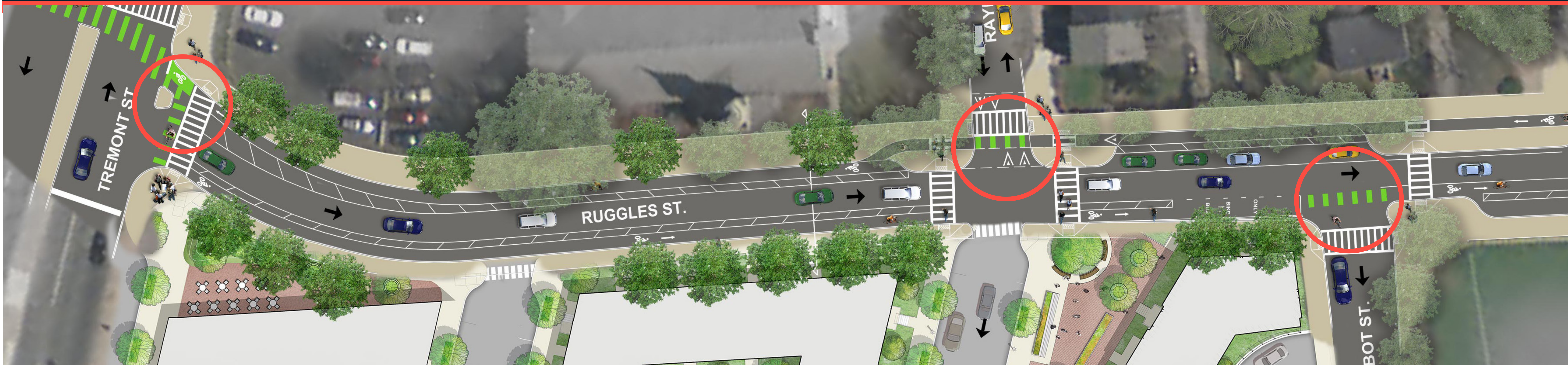
Proposed Improvements: Protected contra flow bike lane, raised and marked crossings, protected buffered bike lanes, two-stage queue box.
