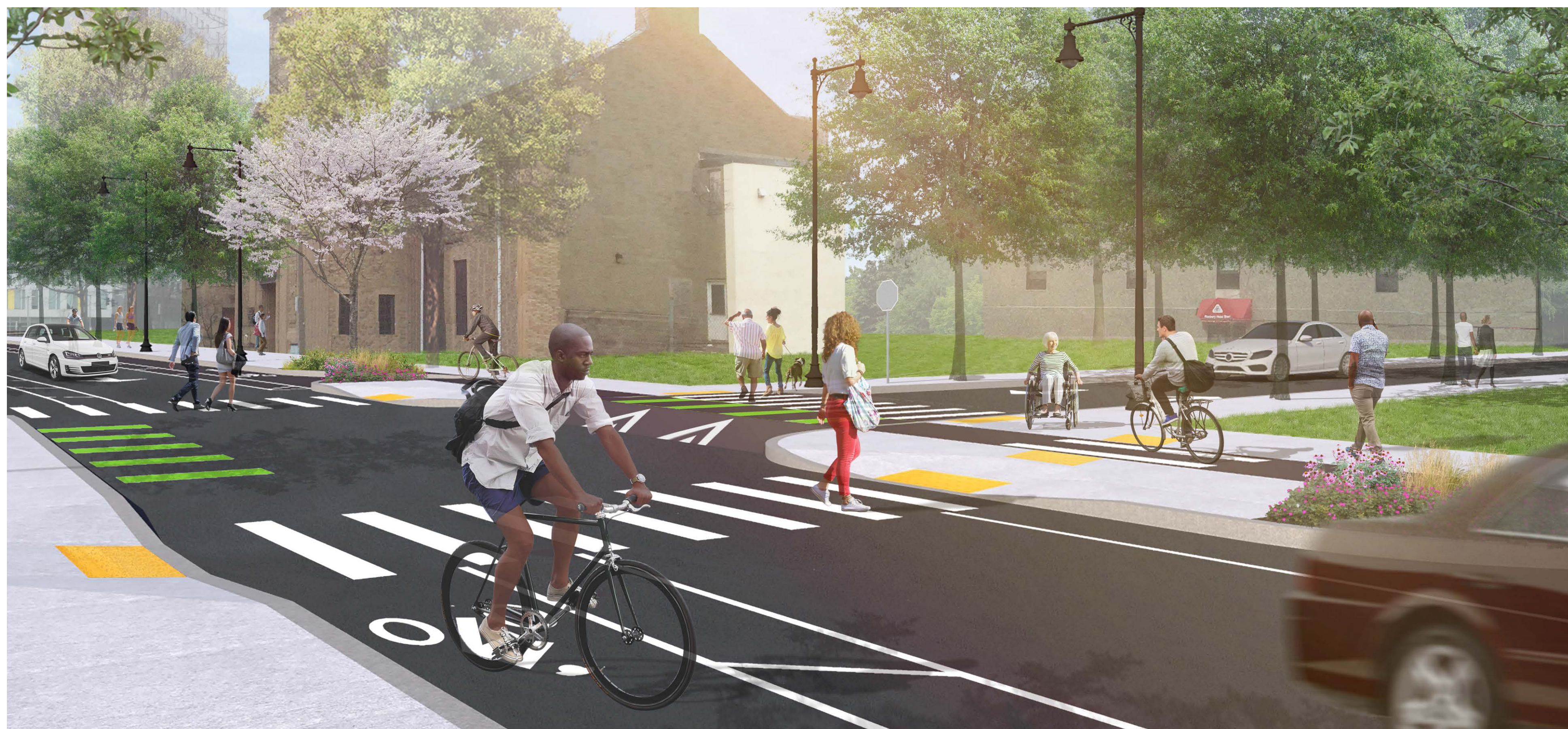
Ruggles Street at Raynor Circle with proposed street improvements (protected contra-flow bike lane, protected bike lane, raised and marked bike crossing (Raynor Circle).
