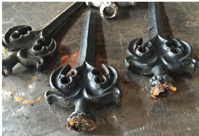
The bottoms of these finials were deformed by welding.
