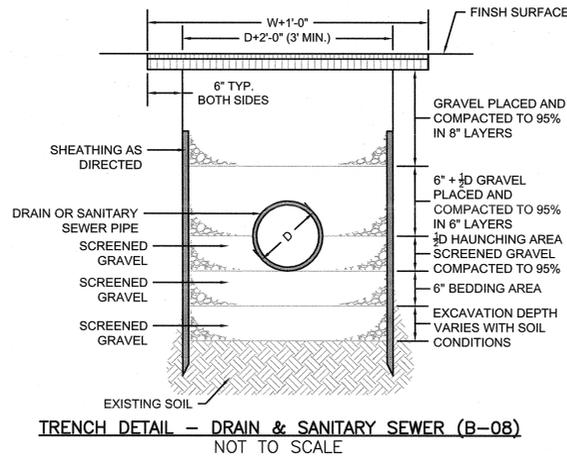
TRENCH DETAIL - DRAIN & SANITARY SEWER (B-08)
