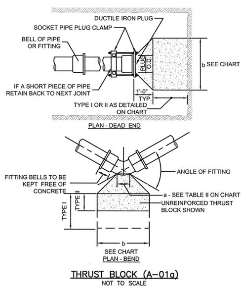
**TABLE I - THRUST - KIPS (WATER PRESSURE = 200 P.S.I.)**
