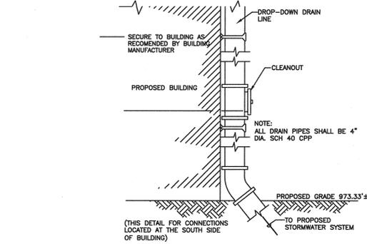
ROOF DRAIN LINE AND DROP-DOWN LEADER JUNCTION DETAIL
