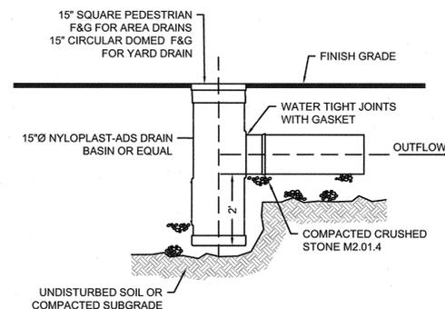
NOTE: STRUCTURE MUST BE ADEQUATE FOR H-10 MIN. LOADING
