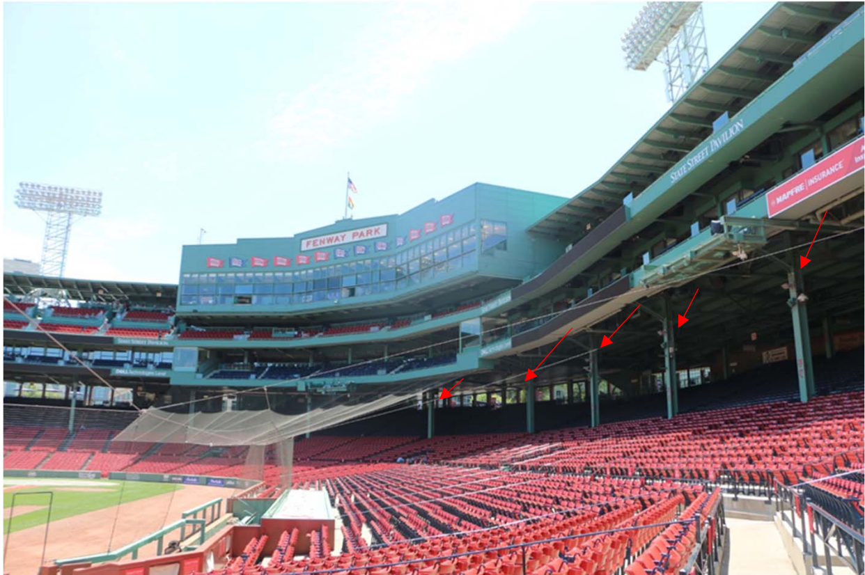
Photo 8: Proposed antenna locations along the east side of the field.
