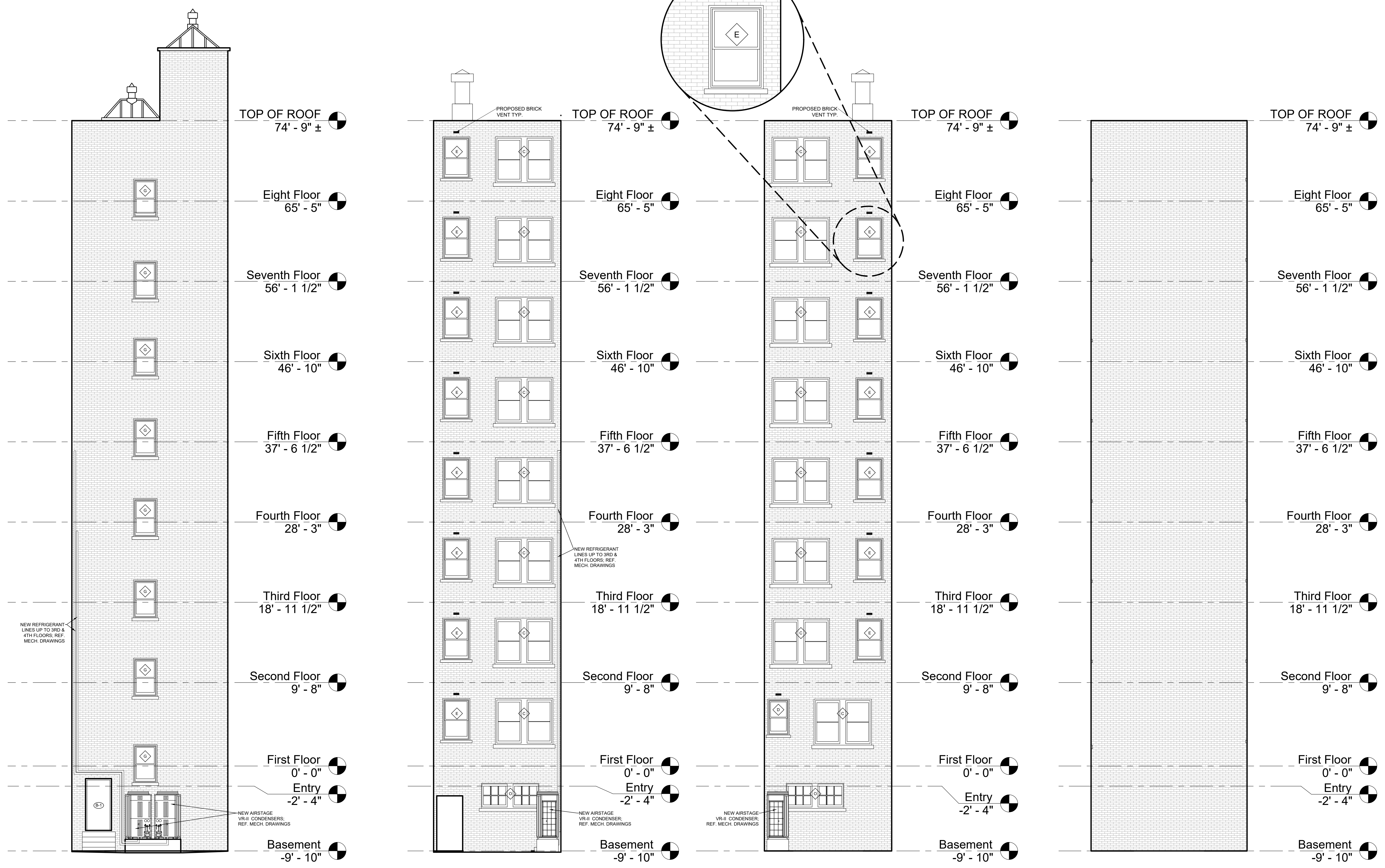
LIGHT WELL #1 ELEVATIONS 1 3/16"=1'-0"
