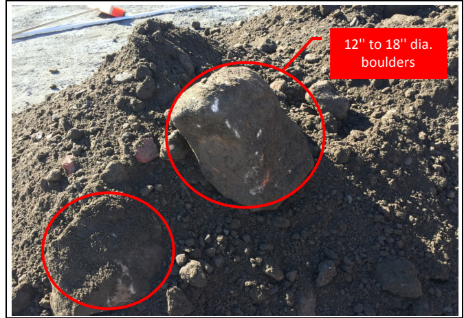
Photo 2 - Boulders removed from test pit.
