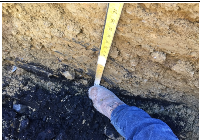
Photo 3 - Possible buried topsoil layer exposed.
