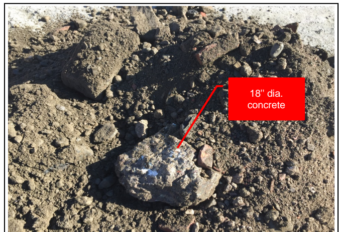
Photo 4 - Debris removed from test pit.
