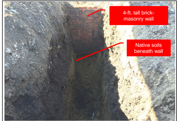
Photo 2 - View of test pit looking west. Buried foundation elements encountered in western half of test pit.
