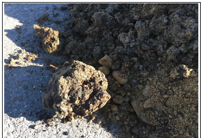
Photo 6 - Debris removed from test pit below a depth of 8 ft. (mostly ash and slag)
