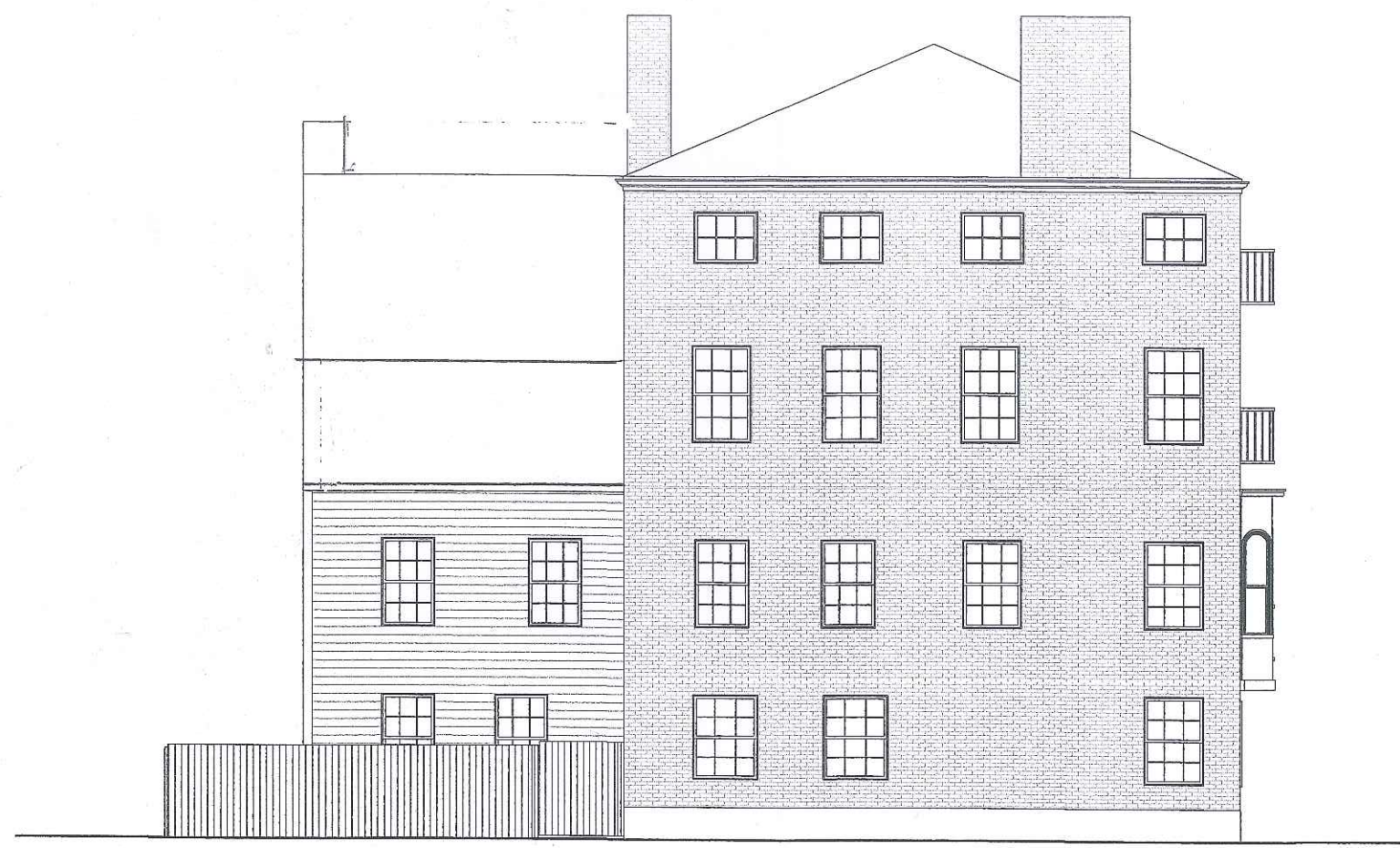
③ SIDE ELEVATION EXISTING 1/4" = 1'-0"
