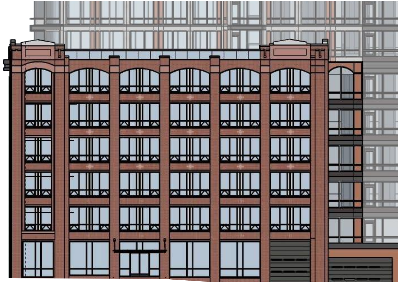
West Elevation - Proposed Parapet - with Telecom Enclosures
