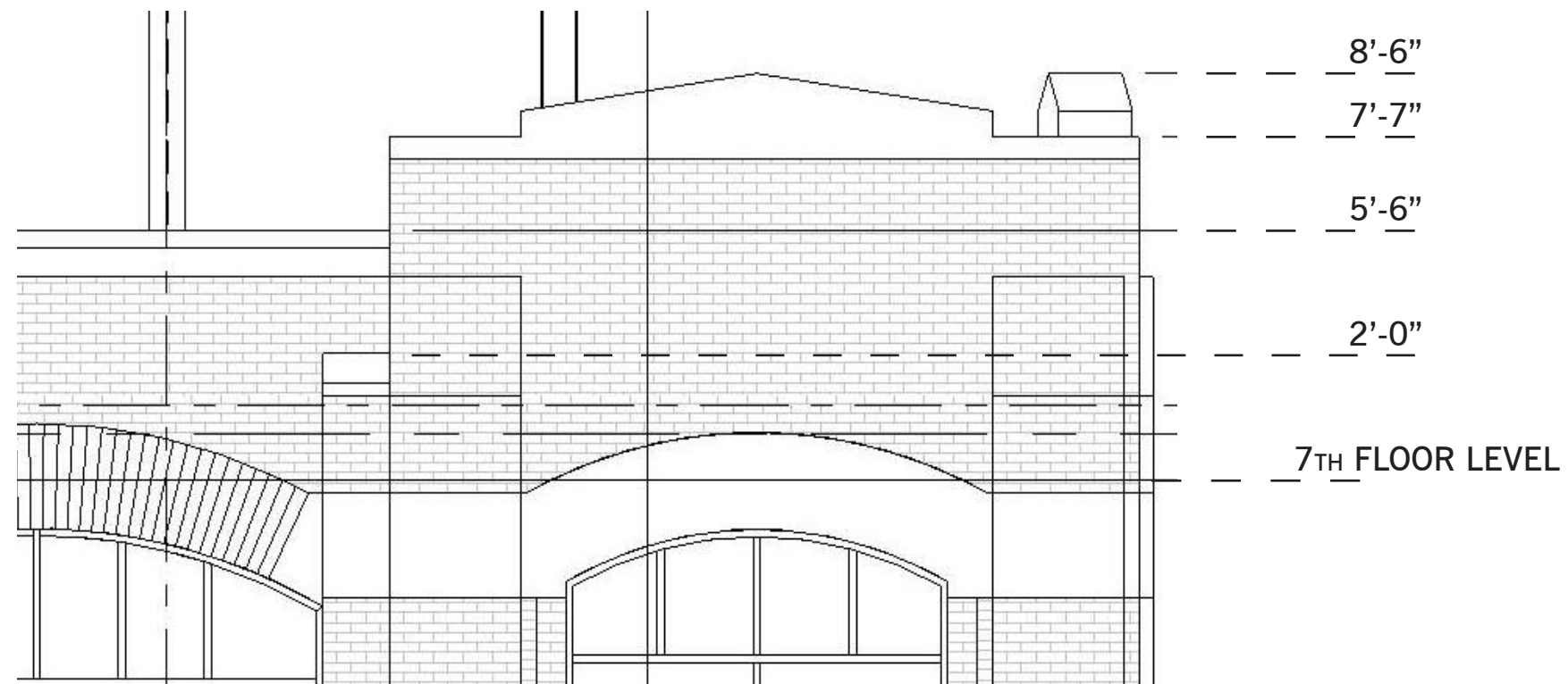
Existing Parapet Profile
