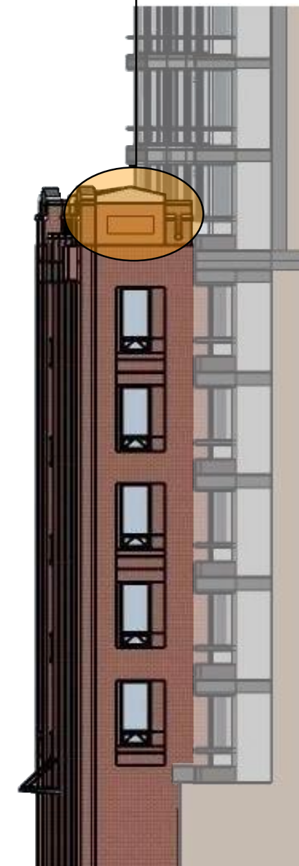
South Elevation - Proposed Parapet - with Telecom Enclosures
