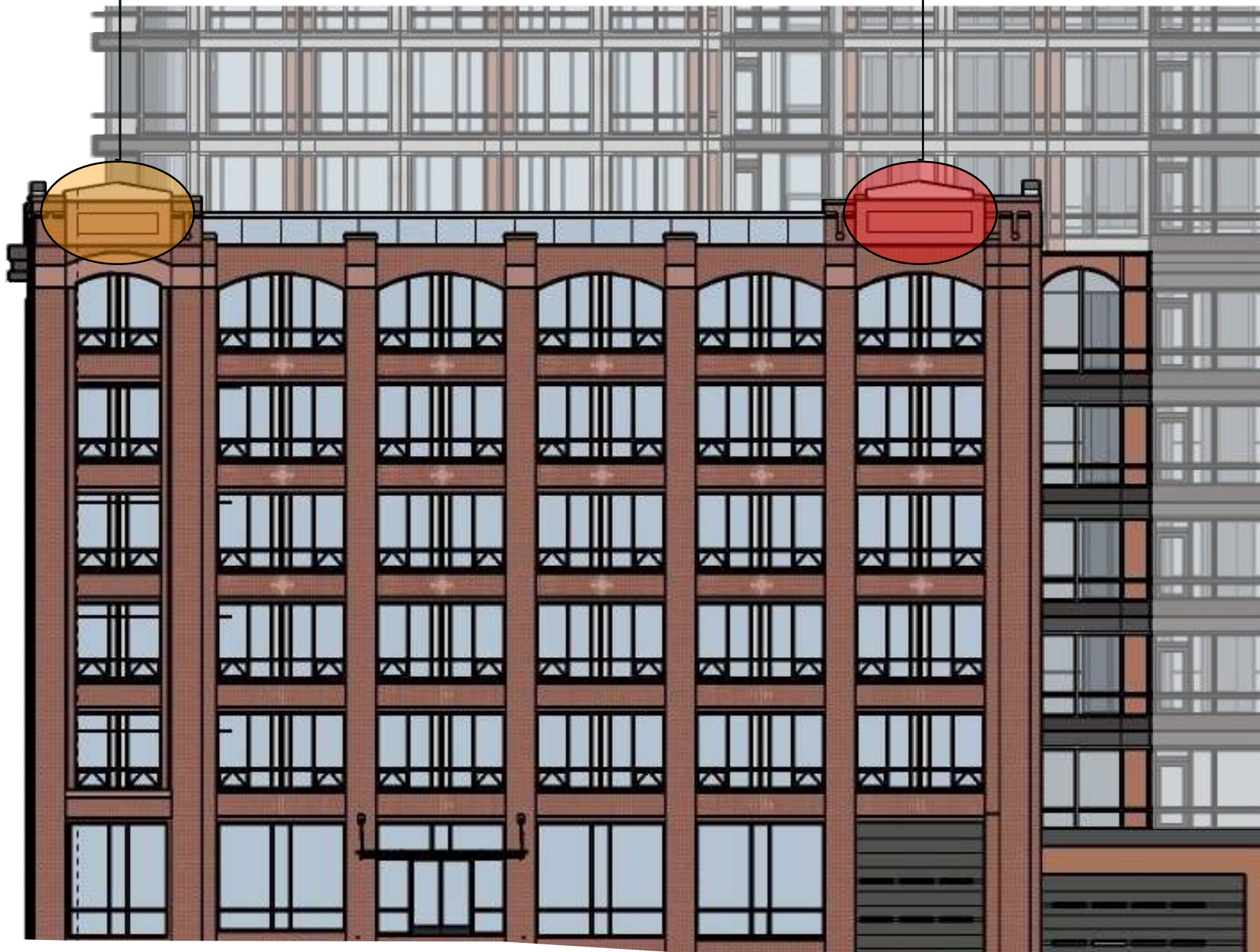
West Elevation - Proposed Parapet - with Telecom Enclosures
