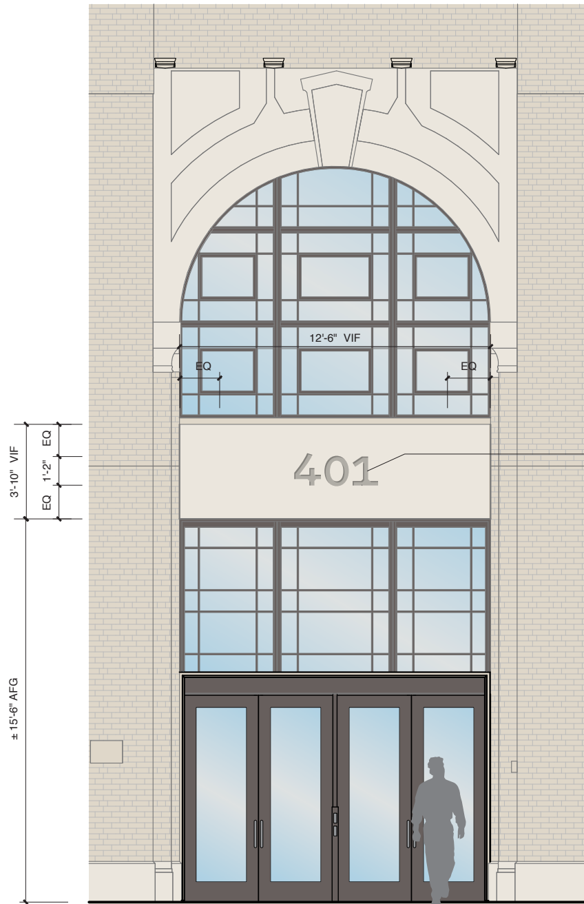
Flat-cut sandblasted letters, 3/4" deep with gray lithichrome infill
