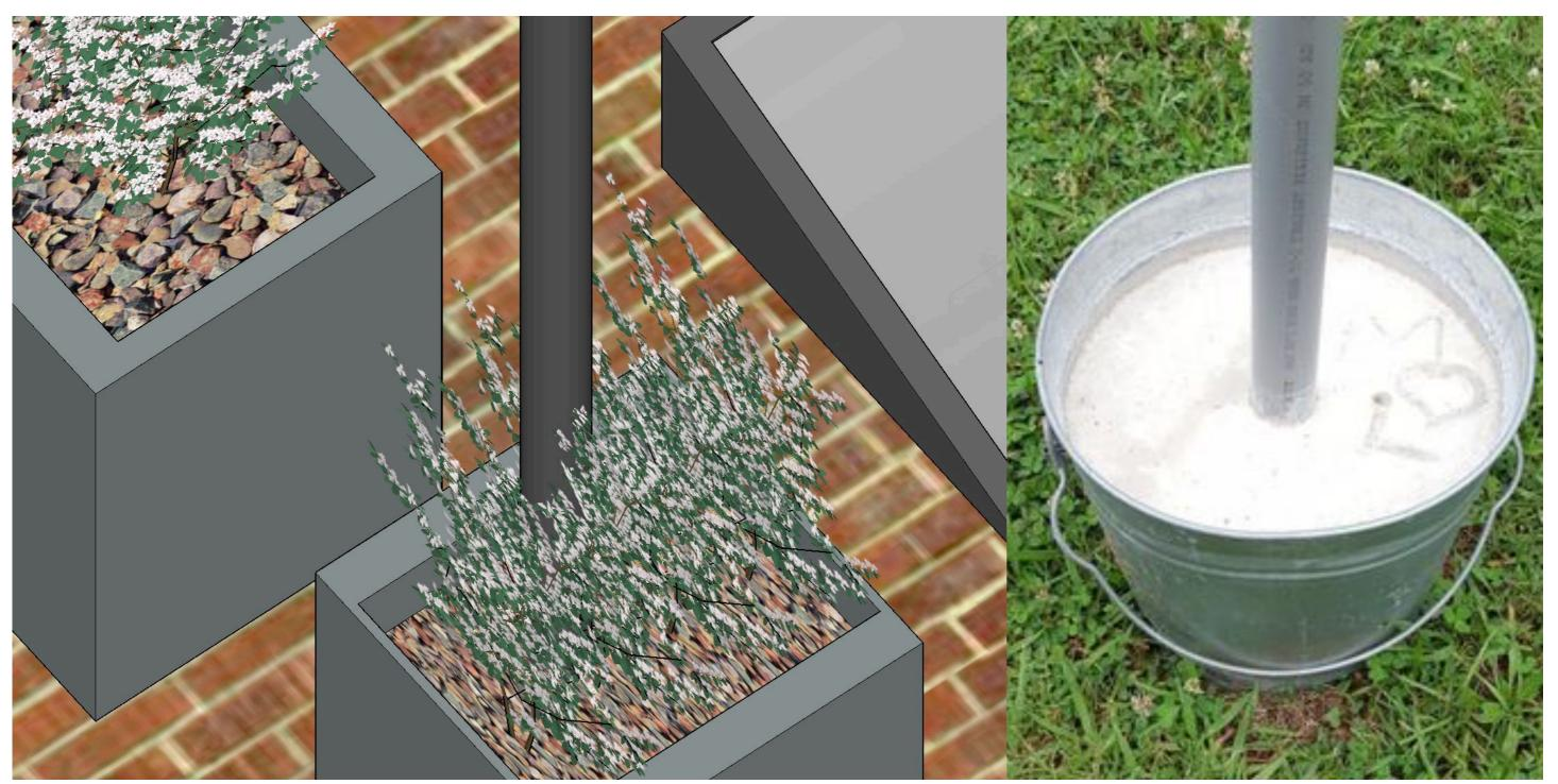
Description: The poles will be able to be removed and a similar cement bucket will be able to receive the pole. The bucket will be concealed by the planter, soil, and plants.
