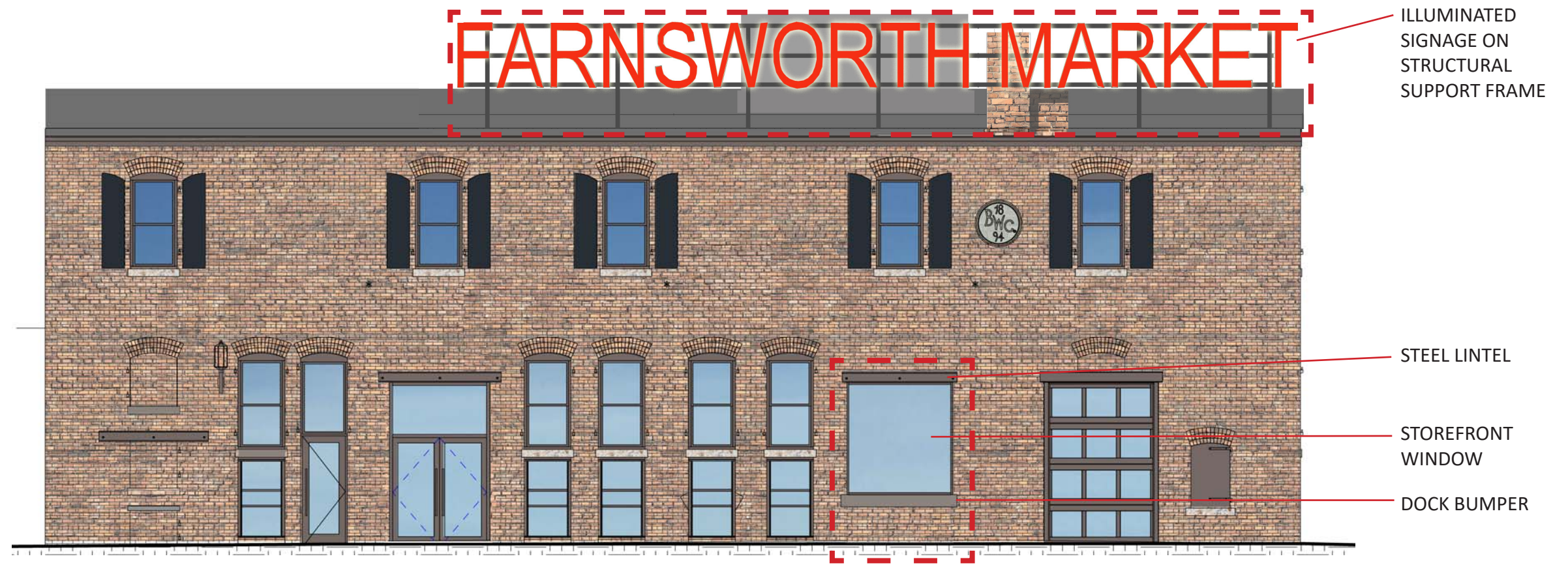
EXISTING CONDITIONS ELEVATION
