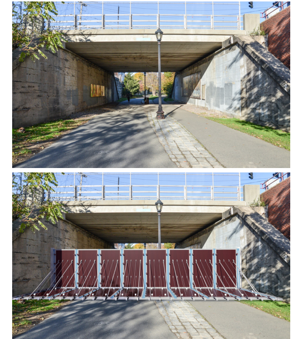
Deployable flood walls, such as the type shown in these renderings of the Greenway under Summer Street, are installed only when a flood is anticipated. They are otherwise kept in storage.
